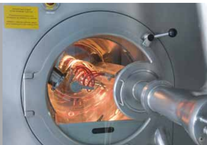
In the hermetically sealed Containment-Facility high-potency substances are processed up to a TLV of 0,001mg/m 3 into tablet form. Photo: Corden Pharma
