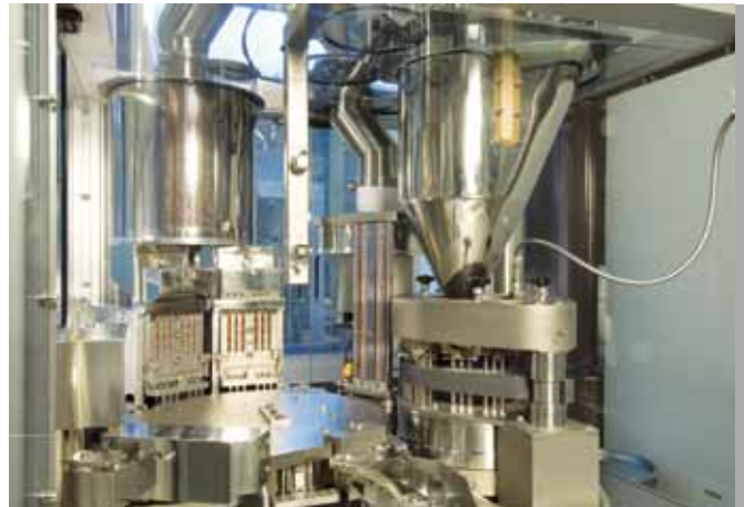
The contract manufacturer has the most modern facilities for tablet production at their disposal. A machine for the production of hard gelatin-capsules is pictured here. Photo: Corden Pharma
